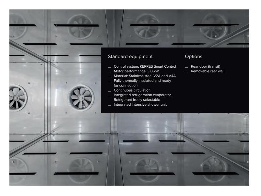
KERRES shower and intensive cooling systems revolutionize production processes by minimizing product throughput times while ensuring a modern and efficient operation. Following the thermal treatment of meat, sausage, and other foods, our systems rapidly cool the goods to the desired core temperature
